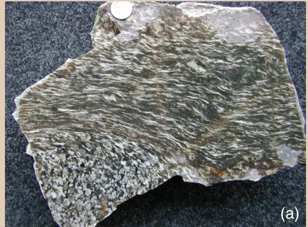
Fig. 11.1: (a) High-pressure shear zones can be observed in natural rocks such as in this meta-quartzdiorite. (b) Shear strains can also be generated in the laboratory, shown by this experimental sample deformed in torsion geometry; the cylinder was twisted twice around its vertical axis
